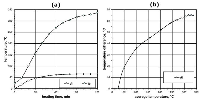
Fig. 7. The temperature difference  $dt$  obtained for the central profile in the sample *B*: a) changes of the parameter  $dt$  and the average temperature of the profile  $t_a$  as a function of heating time; b) change of the parameter  $dt$  as a function of the average temperature of the profile  $t_a$
