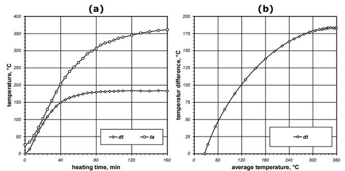
Fig. 4. The temperature difference  $dt$  obtained at the height of the pipe in the sample A: a) change of the parameter  $dt$  and the average temperature of the pipe  $t_a$  as a function of heating time; b) change of the parameter  $dt$  as a function of the average temperature of the pipe  $t_a$
