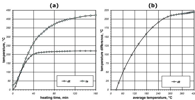
Fig. 9. The temperature difference  $dt$  obtained for one of the profiles in the sample *C*: a) the changes of the parameter  $dt$  and the average temperature of the profile  $t_a$  as a function of heating time; b) the change of the parameter  $dt$  as function of average temperature of the profile  $t_a$
