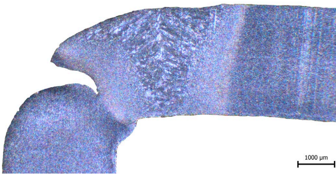
Fig. 4. Cross-section of the EBW welded joint after the bend test
