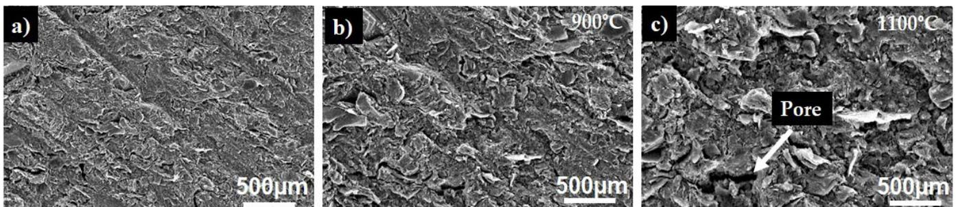
Fig. 1. SEM micrograph of (a) unsintered, (b) sintered at  $900^\circ\text{C}$  and (c) sintered at  $1100^\circ\text{C}$
