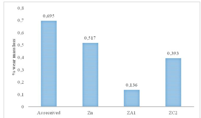
Fig. 10. Percentage wear mass loss of as received, Zn and Zn nanocomposite coatings obtained under dry sliding conditions at load of 5N and speed of 200 rev/min
