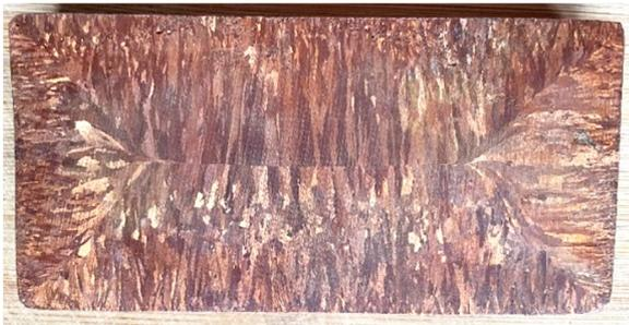
Fig. 1b. Exclusively columnar structure revealed within the copper strand (120 mm x 60 mm); source: KGHM Polska Miedź S.A. – Copper Smelter “Cedynia”
