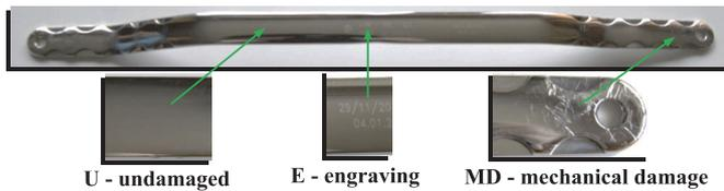
Fig. 1. Sample plates selected for the tests
