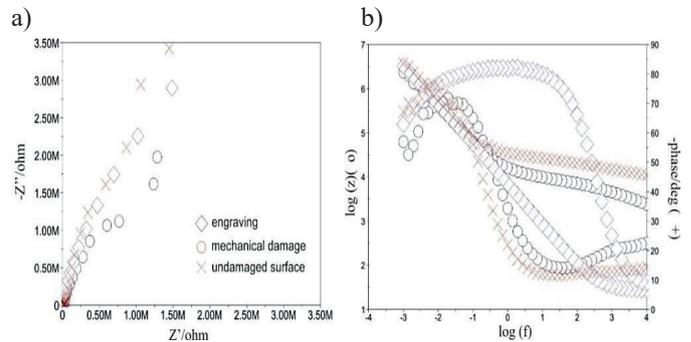
Fig. 5. Sample diagrams for PA plate: a) Nyquist, b) Bode
