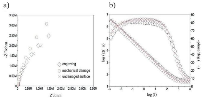
Fig. 4. Sample diagrams for GA plate: a) Nyquist, b) Bode
