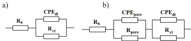
Fig. 6. Equivalent circuit for corrosion system: steel - Ringer's solution
